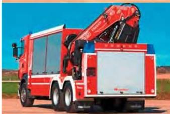
crane, max. 572 kN, ext up to 24.8 m, with remote control
